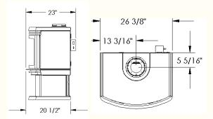
NOTE: When installing the Torino rear vent, a minimum 36" Simpson DuraVent® or Selkirk® snorkel must be used. For detailed installation instructions, please refer to the Owners & Operators Manual.
